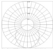
Maximum Candela = 2129.347 Located At Horizontal Angle = 0, Vertical Angle = 0 f 1 - Vertical Plane Through Horizontal Angles (0 - 180)
