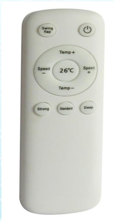
Turn on A/C: Press On / Off button to turn on A/C (long press)
